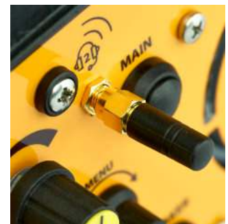
'Wireless Ready' option installed
